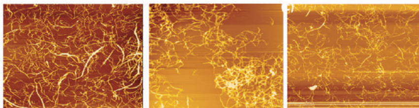
Fig. 6. SPM images of \beta -chitin nanofibers after various passes treatments of chitin slurry
